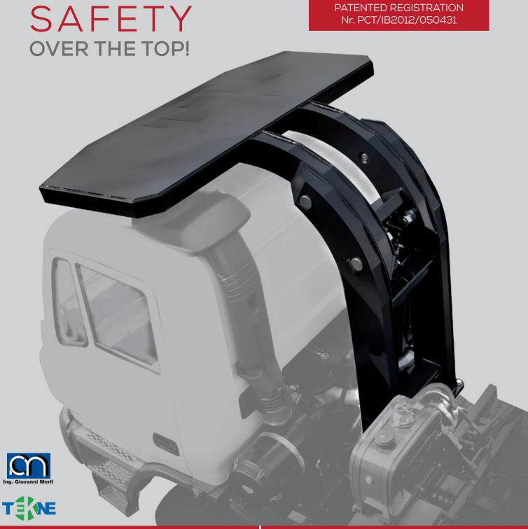
STRUTTURE DI PROTEZIONE PER IL RIBALTAMENTO E CADUTA OGGETTI PROTECTION STRUCTURES FOR **ROLL-OVER AND FALLING OBJECTS**
